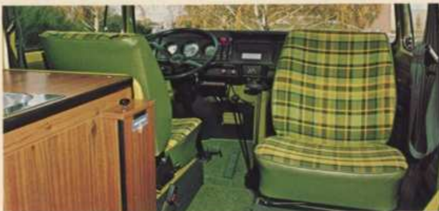
Front passenger seat turns around to become a dining and living room chair.
